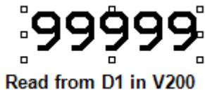
Be sure to select the Modbus tag that is mapped to D0001 in the V200 PLC
