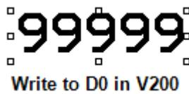
Pressing the data entry 99999 will cause the data entry keypad to appear. Key in a number and press enter
