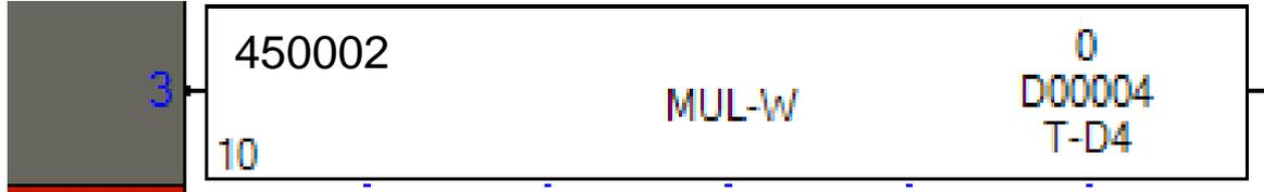
Instead, the value in 450002 must be copied into one of the OIS45E PLUS's registers. This is done using a global task. Select Tasks from the navigation pane.
